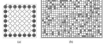
Fig. 9. Large-scale experiments: (a) Rotation problem with 24 robots. (b) Random assignment of 100 robots. Robot *i* moves from S*i* to G*i*.
