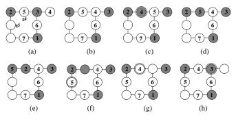
Fig. 5. RESOLVE: Vertices in  $\mathcal{U}'$  are shaded. (a) After robots 1,2 and 3 have planned. (b) Robot 4 swaps with 3. (c) Resolve is invoked (3 was at goal). 4 swaps with 5 and reaches its goal. (d) Resolve called for 3 and 5; 5 swaps with 4. (e) 5 swaps with 2 invoking Resolve again. (f) 5 pushes to its goal; third Resolve is successful. (g) 4's goal is freed; second Resolve is successful. (h) 3's goal is free; first Resolve is complete.
